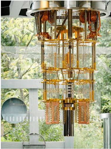
IBM 50Q System: An IBM cryostat wired for a 50 qubit system.
